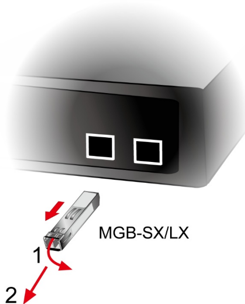
Figure 2-2-5: How to Pull Out the SFP/SFP+ Transceiver
